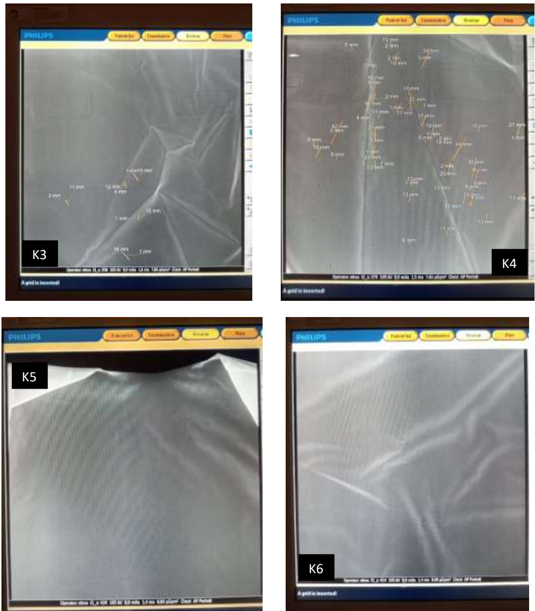
Gambar 4.1 Hasil Radiograf lead apron A
