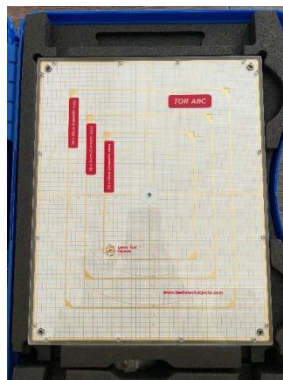
Gambar 3.3 Collimator Test Tool (Universitas Awal Bros, 2024)
